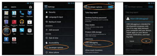
Fig: 3.3.21.1.2 USB Debugging Mode -Android 3.0 - 4.1 X
