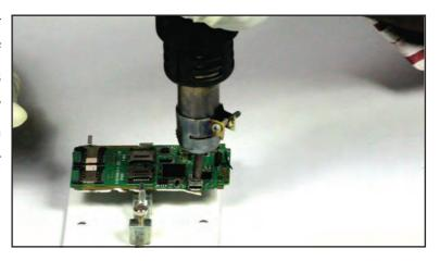
**Step 4**: Now you can see we have remove this charging socket from PCB. This is the lower portion of charging base where it is getting soldered.
