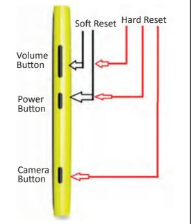
Step 4: Wait for the startup screen booting with an exclamation mark " ! " then release the volume down key
