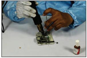
Fig: 3.3.7.1.4 Charging Connector Soldering - Step 1
