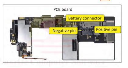
On multimeter it is showing continuity as it is showing multimeter pointer moving forward, it means supply is going from positive to negative. If we change the multimeter probe in reverse direction, multimeter pointer will not move forward. In case pointer is moving forward, it means mobile is having some hardware problem.
