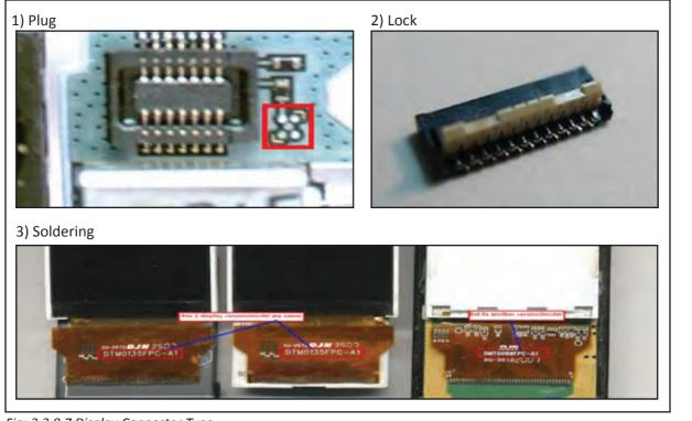
*Fig: 3.3.8.7 Display Connector Type*
