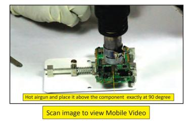
**Step 4:** To resolve the problem of battery discharge or battery blown or auto switch Off, we will use IP and Elmaa liquid to wash the motherboard. After drying the board using hot air gun we will assemble it back properly and after that switch it On.
