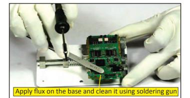
**Step 6:** Now we have assembled ceramic capacitor properly to its location using hot air gun. This is called soldering and De-soldering process.
