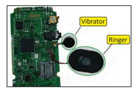
**Step 11:** To remove parts from motherboard set the motherboard on PCB holder
