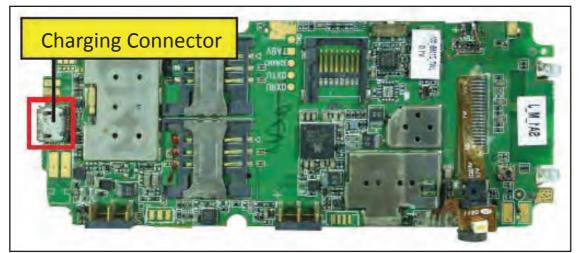
Fig: 3.3.7.1.1 Motherboard - Charging Connector
