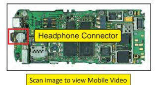
**Step 2:** Headphone track is broken – If the track of headphone is broken then we need to do the jumpering of headphone connector.
