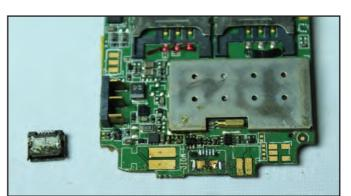
Fig 3.5.7.1.3: Charging Connector and Slot
