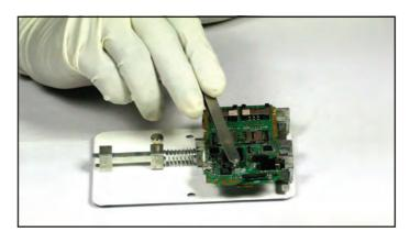
**Step 3:** Fisrt apply flux using tweezers on the component we need to remove. Now switch On hot airgun and place it above the component exactly at 90 degree. Now we can see this component can be separated easily from the motherboard. Remove the ceramic capacitor and keep it in safe place. Now Switch Off the hot air gun.
