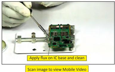
**Step 6:** We will assemble the IC back to its location from where it was removed. Apply heat at base of IC using hot air gun so that base will become thin. It will help us to do the assembly of IC on PCB.
