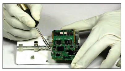
**Step 6:** Now we will apply heat on the base using hot air gun so that solder will melt and become thin. Once it melts we will place the charging socket back to its location.
