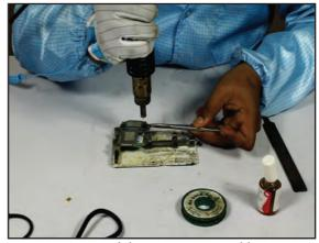
Fig: 3.3.7.3.2 Headphone Connector Soldering - Step 1
