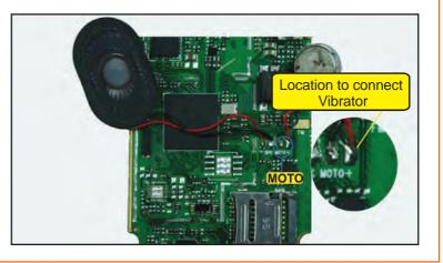
**Step 25:** Be careful while soldering the wire, always connect positive wire with positive pin and negative wire with negative pin. Location for positive is marked with "+" where as negative is marked with "-" sign.
