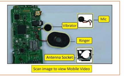
**Step 24:** Now we will connect speaker. er. Location from which speaker was taken out having text marking SPK which indicates speaker location next to that location we can see text MOTO, it means Motor Vibrator. This indicates place to connect Vibrator. Text marking helps us to locate part's location on the motherboard. Now we will place both the parts at their respective locations.
