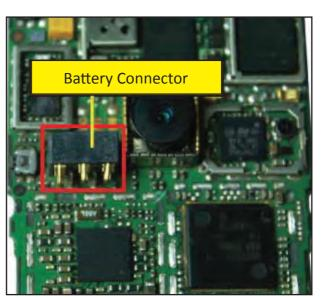
Fig: 3.3.7.2 Battery Connector
