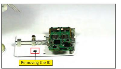
**Step 5:** Now inorder to place the IC back, we will apply flux and with the help of soldering gun try to do the re-soldering. At first we will clean all the legs then after apply flux on IC base and clean it properly.
