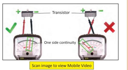
Step 4: We will test the continuity of these components; all these components during test process will show one side continuity. In case any of these components are showing both side continuity this means that particular component is faulty and we need to replace it. After replacing the component probably problem will be resolved and we can turn dead mobile to working mobile phone.
