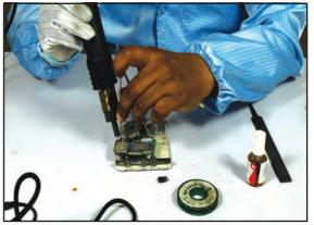
Fig: 3.3.7.3.3 Headphone Connector Soldering - Step 2
