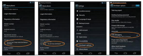
Fig: 3.3.21.1.4 USB Debugging Mode -Android 3.0 - 4.1 X
