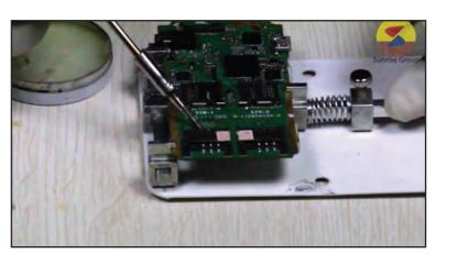
**Step 5:** Now we will use another end of jumpering wire to connect broken track. You can see silver base on this track. We will clean the base with the help of solder gun and then apply flux to do the soldering of another end of the jumpering wire. Here we can see we how we did the jumpering from SIM tray pin to base of track. This process is called jumpering
