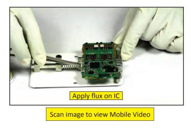
**Step 3:** Now we will remove this IC using hot air gun. As you can see I have hold the hot air gun at 90 degree angle on top of the IC. Now rotate the hot air gun in anticlockwise direction on top of the IC to make sure heat is applied on all sides of IC so that it will become easy to remove it. You can see I have removed this IC and kept it aside.
