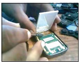
Fig: 3.3.7.9.2 Display Strip Assembly
