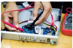
Fig 5.2.1(b): Connec ng data port on the panel board
