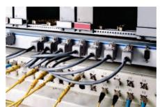
Fig 5.2.1(e): Connec ng cables to DVR
