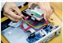
Fig 5.2.1(c): Placing hard disk within DVR
